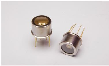
The P11120-201 is a cooled type infrared detector that provides high sensitivity in the 5 μm spectral band by employing our unique crystal growth technology. It has a PN junction that ensures high-speed response and high reliability. D\* is improved as a result of cooling, enabling higher-accuracy gas detection. Handling is easy because it is a TE-cooled type that uses a TO-8 package.
