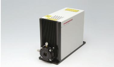
The Pulsed QCL Module is a compact module containing a TO-8 can packaged pulsed DFB quantum cascade laser, pulse driver and TEC controller. The module can be easily and remotely controlled via Ethernet connection.
