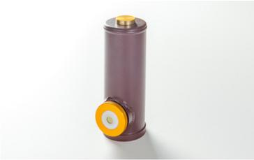
This is a Type II InAs/GaSb superlattice infrared detector with the spectral response range expanded to the 14 μm band. The spectral response range has been expanded using Hamamatsu unique crystal growth technology. This product is an environmentally friendly infrared detector and does not use mercury or cadmium, which are substances restricted by the RoHS Directive. This is a replacement for previous products that contain these substances.
