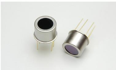
The P12691-201G is an infrared detector that provides high sensitivity in the 8 μm spectral band by employing our unique crystal growth technology and back-illuminated structure and by integrating a lens. It has a PN junction that ensures high-speed response and high reliability. Handling is easy because it is a TE-cooled type that uses a TO-8 package. Typical applications include gas analysis such as NOx, SOx, and H2S.
